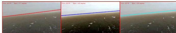
Fig. 5. MPI GPU-accelerated processing of video data for horizon recognition in real-time mode
